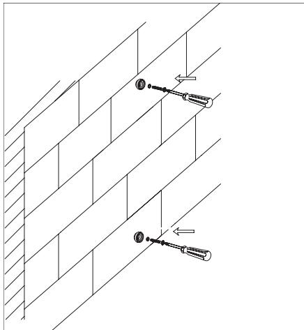
1. Mark the position on the wall according to the dimension drawing. Drill holes on the wall as per size of wall screw set provided. Fixed the wall screw set into the holes. take out the screw and leave the plastic plug in the holes.
