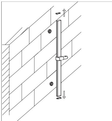
3. Remove the decorative cover on both sides, fix the sliding bar to the wall
