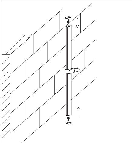
4. Fix the plastic clip to the fixed ring inside the slide bar at the right position. Install the decorative cover back to the slide bar.
