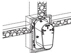
Connect the hot(left) and cold(right) water supply using applicable sealing practices. Remove the cover on concealed box and test for water security with the mixer in both open and shut positions.
