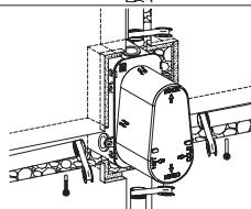
Either, sheet around the concealed box with fibre cement sheeting or backfill the exposed channels ready for tiling. Ensure tiles are cut as close to the concealed box as possible;
