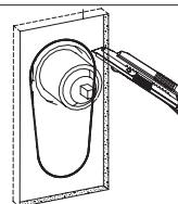
Cover the reserved area with a tile, which should be primarily cut with 2 holes as per the dimension of domes, and size of concealed box.
