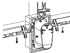
Either, sheet around the concealed box with fibre cement sheeting or backfill the exposed channels ready for tiling. Ensure tiles are cut as close to the concealed box as possible;
