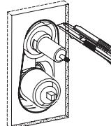
Cover the reserved area with a tile, which should be primarily cut with 2 holes as per the dimension of domes, and size of concealed box.
