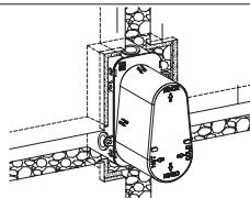
Connect the hot(left) and cold(right) water supply using applicable sealing practices. Remove the cover on concealed box and test for water security with the mixer in both open and shut positions.
