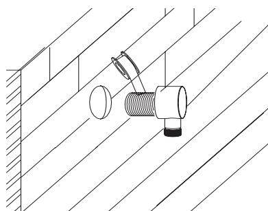
**2.2 Installation of valve body.** Assemble the body with s-shape connector by fastening the nuts with wrench. Make sure the rubber sealing gaskets are inside the nuts.
